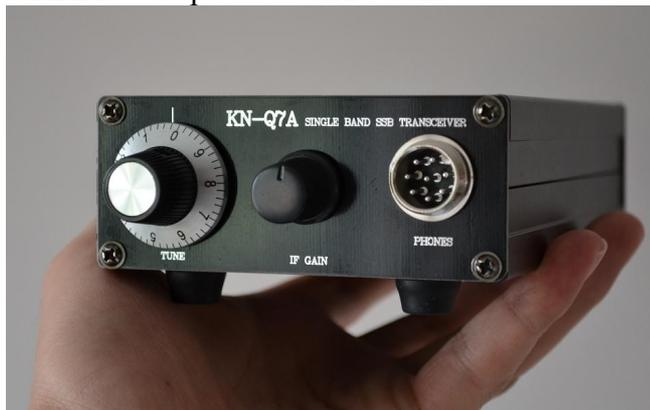
The KN-Q7A single band SSB transceiver kit was designed specifically for the worldwide market by BA6BF, and kitted by BD6CR/4. As the upgraded version of the popular KN-Q7 (more than 500 kits were sold worldwide), the KN-Q7A has an improved circuit design and component selection, which makes it an ideal candidate for field operation, back pack and emergency use.
