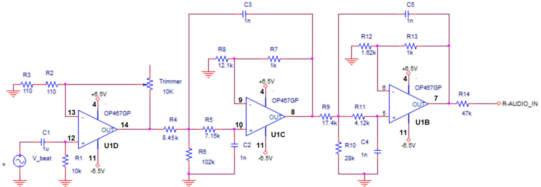
The amplification is set by the trimmer and the filtering modules determine the maximum bandwidth frequency around 15 kHz..
