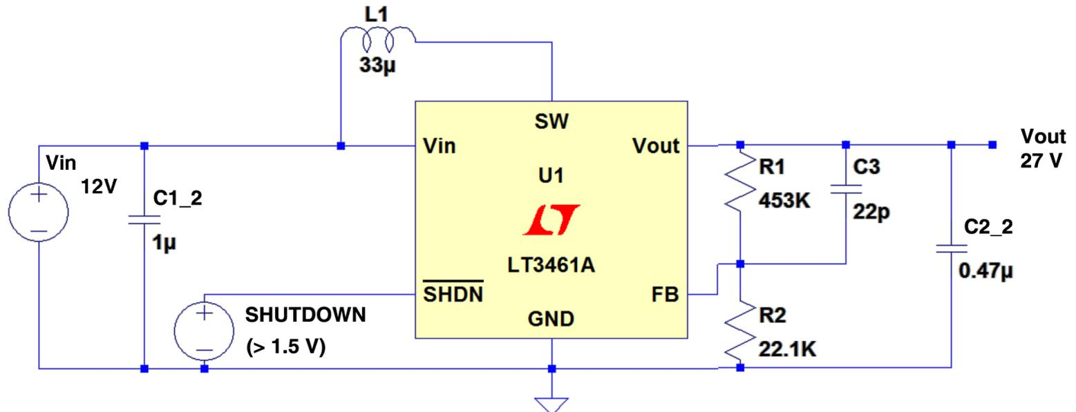
Circuit is a DC-DC step-up converter. LT3461A device switches at 3MHz. This high switching frequency enables the use of tiny, low cost and low height capacitors and inductors.
