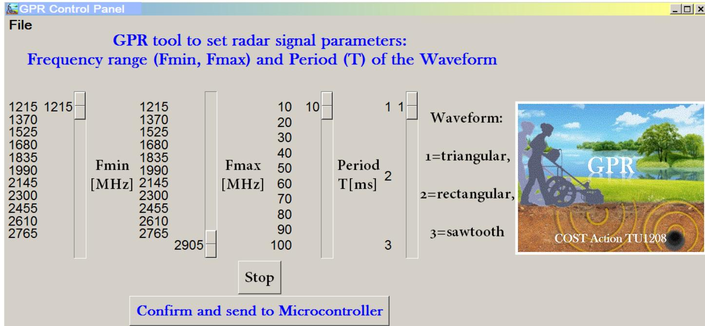
Figure of the graphical interface dedicated to the FMCW GPR prototype control
