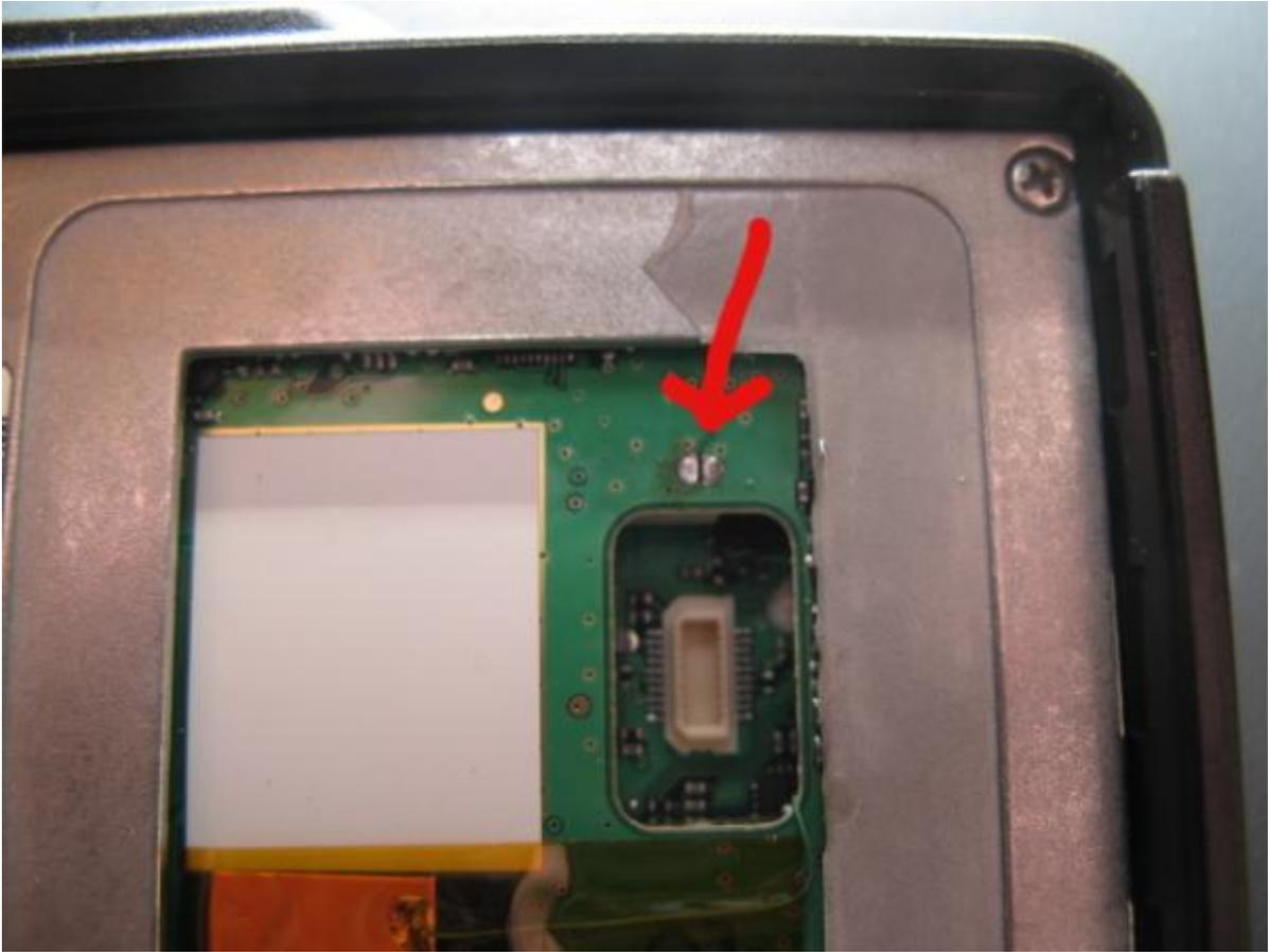
Make sure you clean off ALL the residual adhesive. Don't try to put back the cover that you took off, as it will be badly deformed and you will have lost some of the adhesive. Yaesu gives you several extra covers in the bottom of the box, so use a new one. **This is important to preserve the waterproof integrity of the radio!**
