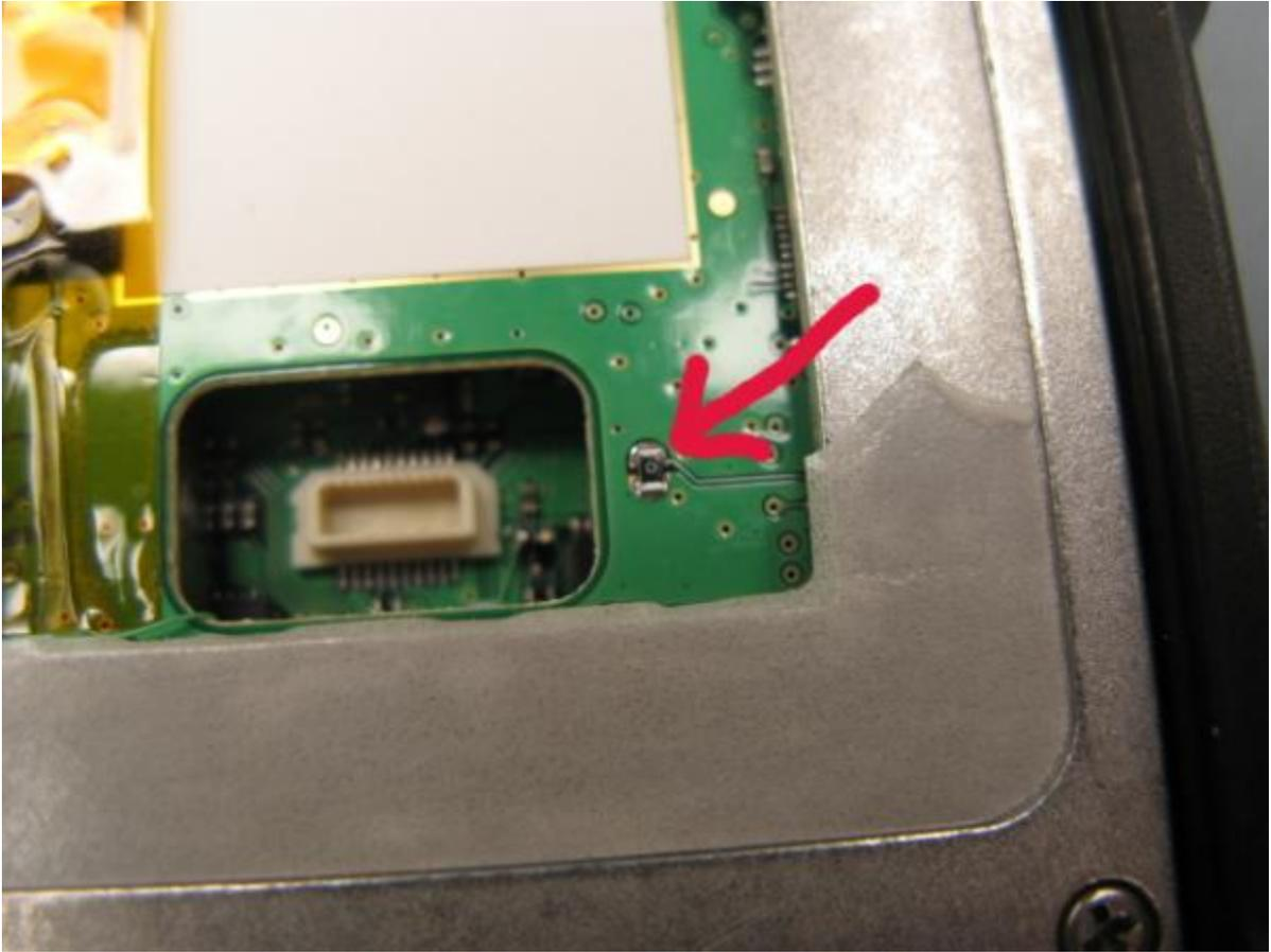
All you have to do is carefully remove this resistor. I have a fine tip for my solder station for little work like this:
