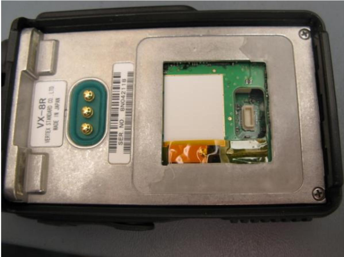
To mod the radio for out of band TX, locate the only resistor visible on the board, just to the left of the bluetooth plug:
