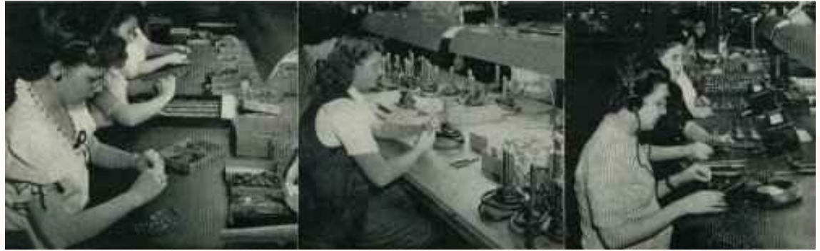
Left to right: assembling needle chuck to crystal element; servicing microphone cables; testing phonograph pickups
