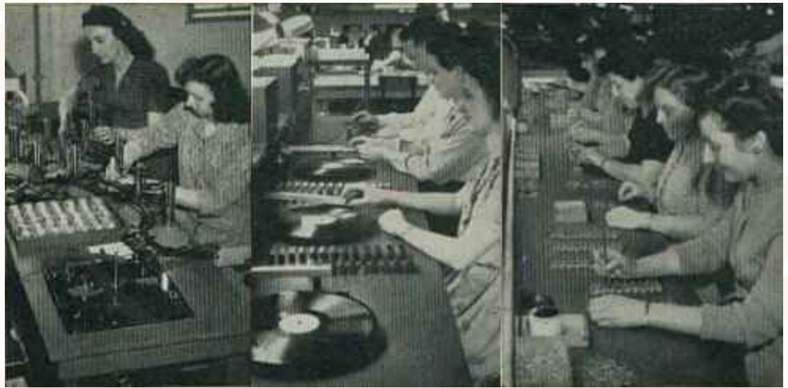
Left to right: Testing Astatic microphones, testing crystal cartridges, cementing damping pads in cartridge housings
