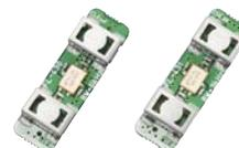
6 kHz or 3 kHz roofing filter can be used. The roofing filters reduce interference from strong nearby signals.
