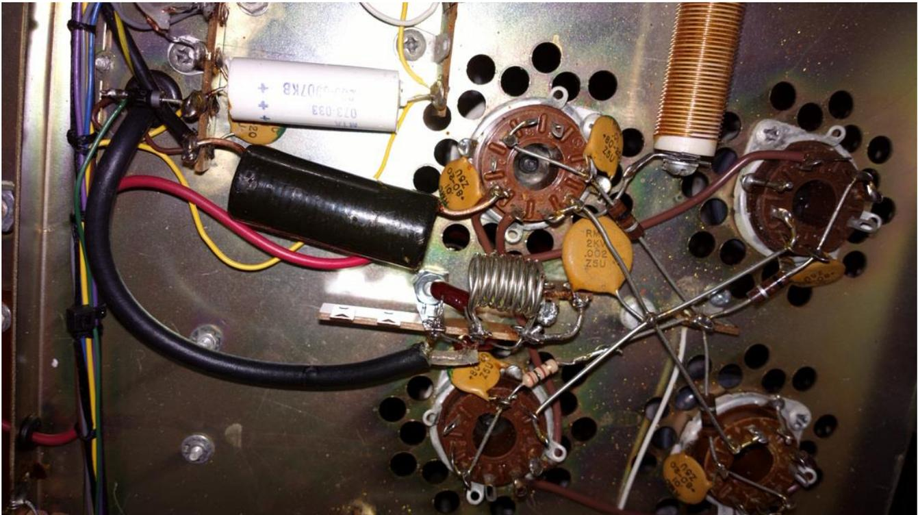
The sites predicted that this filter would roll off before the frequency reached 10 meters, and interestingly, after my 930S tried repeatedly to tune up on 10 meters, the inductor was hot.
