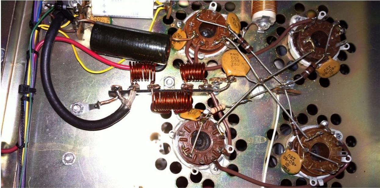
This filter worked very well, allowing my Kenwood tuner to work with all the bands from 10M to 80. The only problem was that the air-core design resulted in significant attenuation of the input signal. I lost at least 50 watts output.
