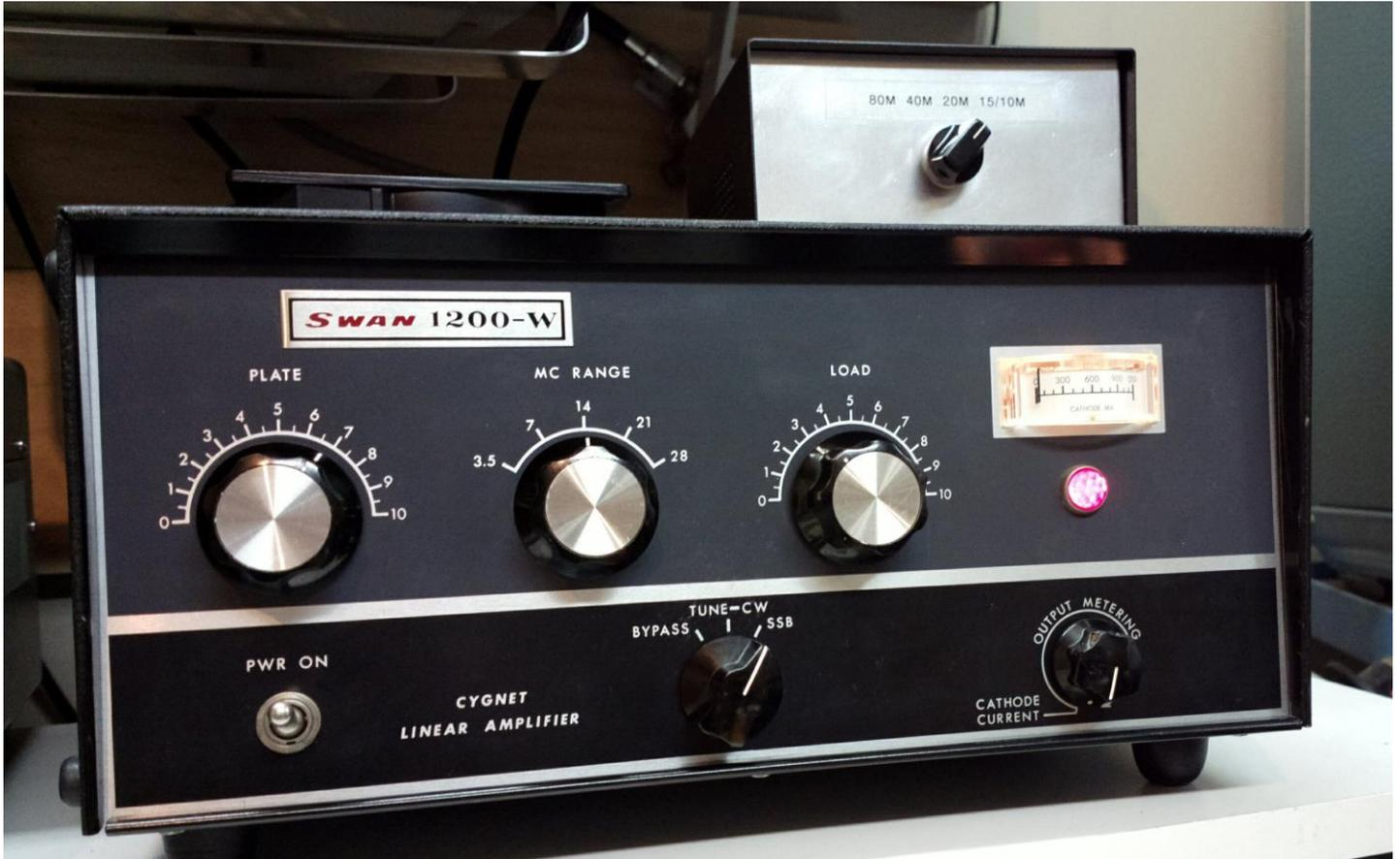
This amp is a prime candidate for mods, because it has lots of room inside. It produced about 400 watts PEP out of the box with the 6JE6's that came in it. Only one tube was “down” a little, and it was a Realistic brand tube.
