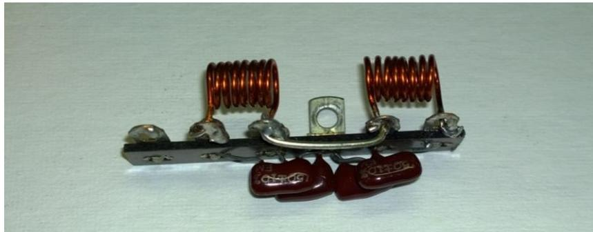
I bought the filter below from a Russian eBay seller, R3KB04. This is a 2-section T-Filter, especially well-suited for low impedances. I was testing it in this picture. Note the cutoff frequency, marked on the filter. This worked so well, it became the "one to beat". My plan is to install this in another small linear that I have that also lacks an input filter.
