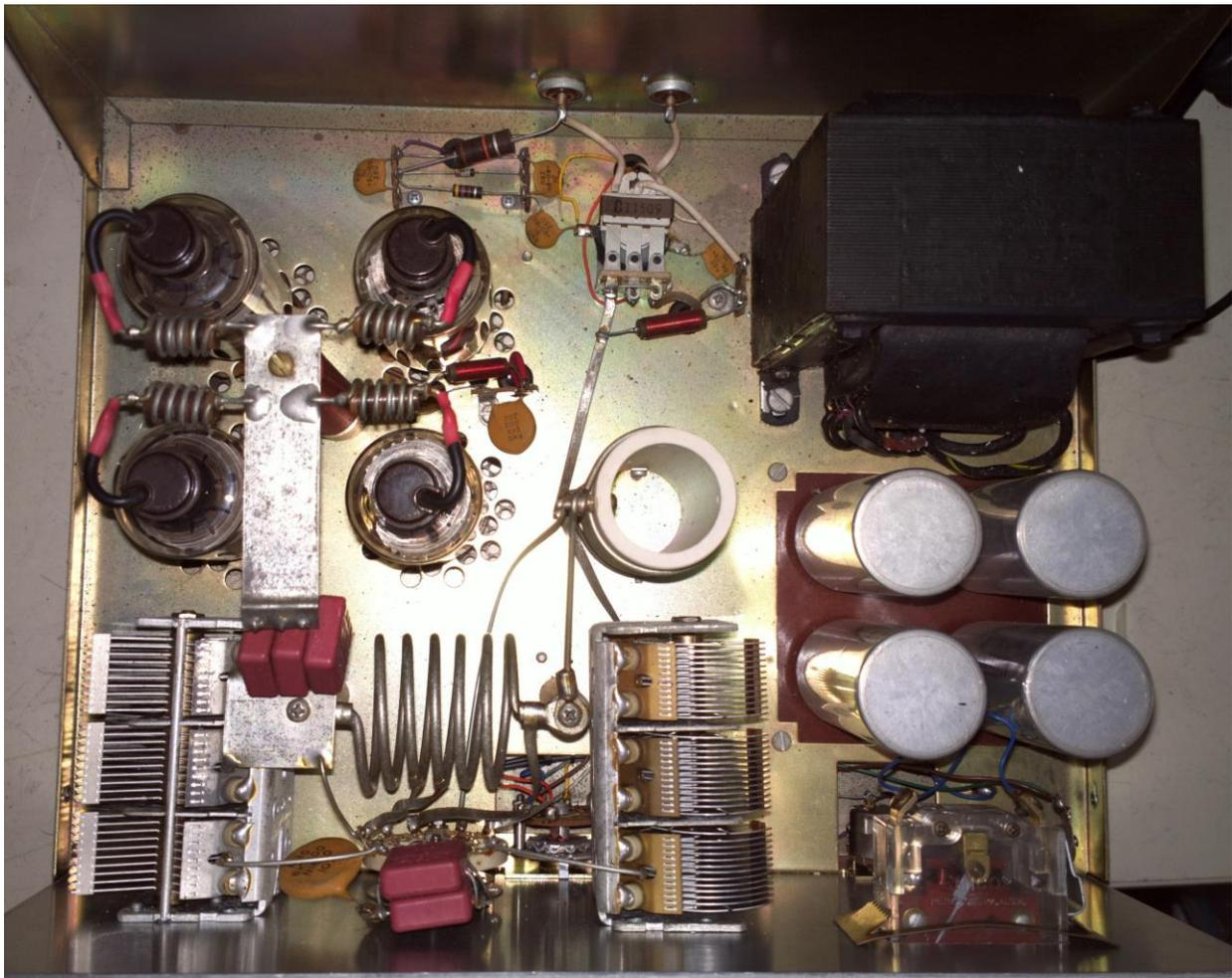
I thought long and hard about putting a filter network on the top of the chassis between the switching relay and the tank coil. A hole and grommet could be put in the deck, and the filter could go in a small metal box. However, voltages run high there, and I was worried about arcing, feedback, etc. I decided that under the deck was best.
