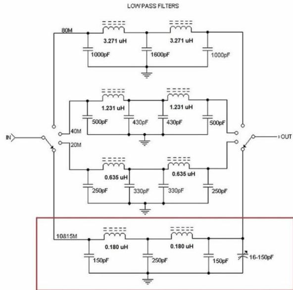
Note that the 10-15M filter portion of the Palomar LPF uses air inductors, and the rest are toroidal. The picture below shows my copy of this filter. I didn't have the correct adjustable trimmer in my parts bin, so I measured the value of the trimmer in the Palomar filter using my LCR and installed a fixed capacitor instead. This worked, but not as well as the one in the Palomar LPF, and it reduced my output. So, I decided to keep looking
