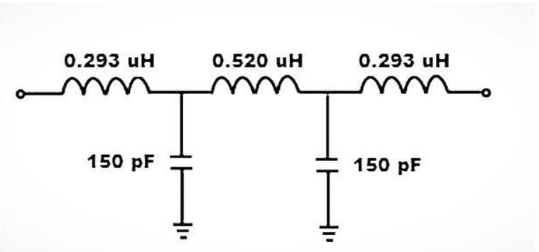
The parts values you see in the schematic aren't marked on the filter. I used my new CEM LCR to find the values. I unsoldered one end of each toroid to accurately read its value. This filter worked great in my 1200-W, but the large diameter coils made it too tall to fit under the deck. I decided to duplicate their filter using air-core coils.
