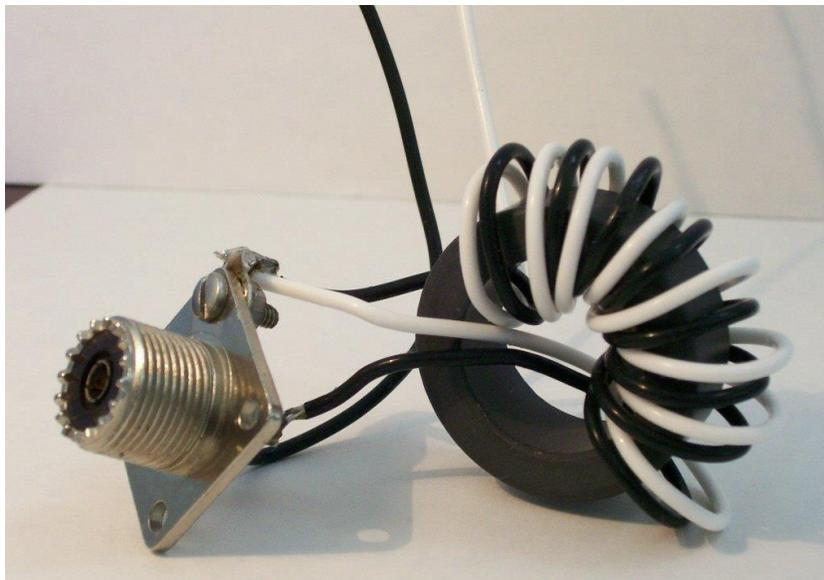
The hardest part was winding the wires tightly enough so that the balun would fit. At one point, I considered installing metal stand-offs and long bottom screws to shift the amp’s bottom plate downward to create more space underneath. I even bought some stick-on lead shielding to try to reduce interactions between the chassis and the balun.
